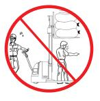
Don't place any part of your body in any moving part of the truck to avoid being clamped.
