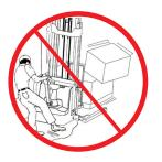
Don't use the truck on slippery road surfaces. (such as road surfaces with oil stain or residual snow or those frozen ones )
